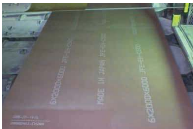
Typical appearance of primer-treated Standard Series plate (EVERHARD-C500 (JFE-EH-C500))
